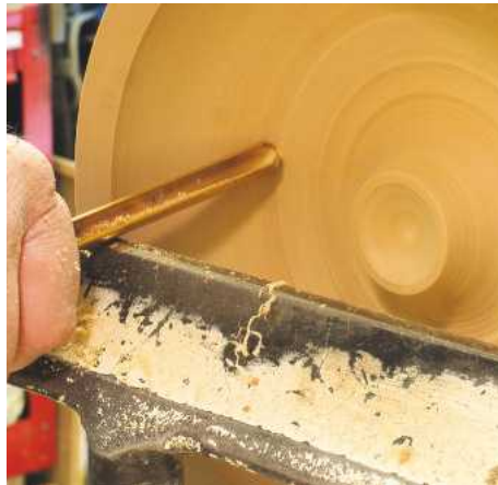
▲ Pic.11 Tooling the curve in the bottom well is not easy. A 10mm gouge is first worked down in the same way that you would turn a normal bowl
